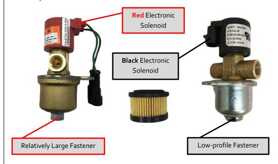
The system manufacturer recommends that you replace the filter for the above lock-offs every 15,000 miles or at least once per year. It is important that you use the correct replacement filter. Below noted are the correct part numbers of each filter repair kit.
