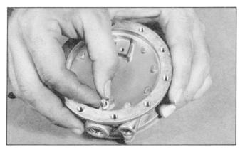
21. Lubricate the Pin Valve (10) with petroleum jelly and insert through hole in the Washer Retainer Seal (14) and Lip Pin Seal (9). Rotate head of Pin gently in a circular motion to ease Pin into place through the Washer, Lip Pin Seal and Body (7) housing.
