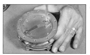
4. Remove Screw (4) retaining Valve Spring (11).
