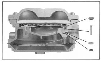
9. Cutaway shows assembly of Valve Spring (11), Valve Seat (19), Valve Operating Pin (10), Seal Retaining Washer (14) and Pin Lip Seal (9). Note that removal of Valve Pin allows retaining Washer to be removed through the ¼" NPT opening labeled "Out."
