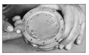
23. Valve Seat (19) shown with aluminum side up ready to be placed on jet.
