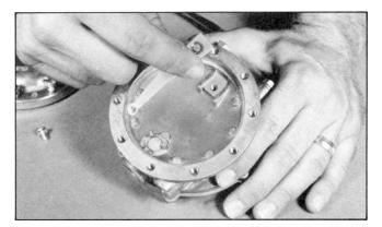
25. Spring (11) ready to be fastened in place. Be sure the arc in the center faces upward (see illustration in step 26 below).
