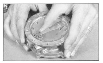
27. When Spring (11) is in place, lift it slightly to ensure it can move freely.
