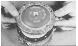
31. Insert two Screws (17) opposite each other in the "Fuel In" cover and place on Gasket (15). Thread the two Screws (17) through the gasket and into the Body (9).
