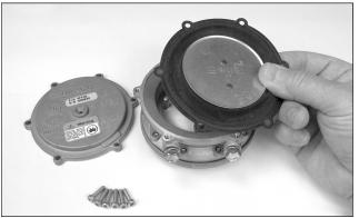
13. Remove Cover (2) and diaphragm (3). Clean covers, body and metal parts as necessary with a safety solvent and dry prior to reassembly.
