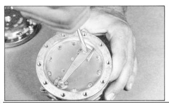
26. Replace Spring (11) and fasten in place with Screw(4). Align the tip of Spring (over valve) and centerbetween the 3 guide fins as shown in illustration.Tighten Screw 28-32 in-lbs. (3.2-3.6 Nm)
