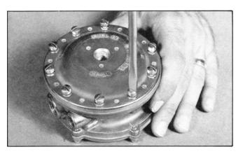
33. Tighten Screws (17), alternating from side to side on opposite sides of the cover until all screws are solidly set. Torque to 60-70 in-lbs. (6.8-7.9 Nm).
