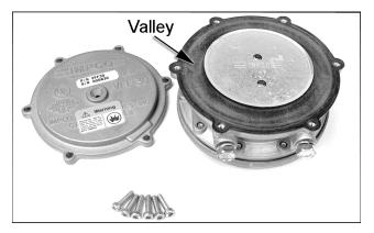
35. Turn Diaphragm (3) so the <u>gasket side is down</u> (see illustration on page 2) place on the Body (7) and rotate to position so the screw hole pattern aligns with the holes in the Body (there is only one position in which the holes will line up).
