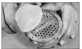
28. Insert Screen (12) and Filter (13) into recess.
