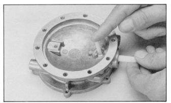
18. Coat the Pin Insertion Tool with petroleum jelly and push the Seal (9) through the Holder and into the Seal recess of the VFF30 Body (7). Look through the fuel port to ensure the Seal is seated in the seal recess and that the groove in the seal is visible.
