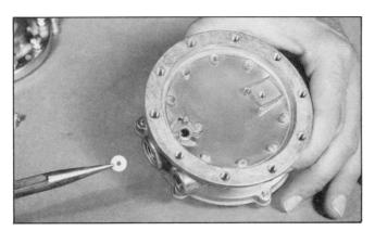
19. Use needle nose pliers to hold the Seal Retainer Washer (14).
