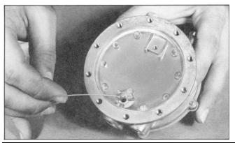
11. Using the same hook, remove the Pin Seal (9) through valve jet.
