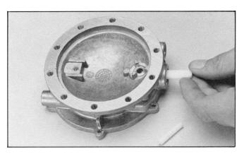
17. Place the holder in the up position and slide the Holder and the Seal (9) into the Body (7) of the VFF30. Looking through the fuel port, position the Seal above the cavity of the seal recess.
