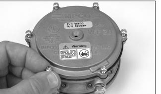
36. Place Cover (2) in correct position and insert Screws (1).
