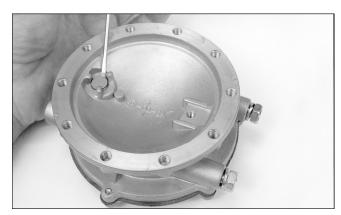
6. Using a small flat head screwdriver, remove Valve Seat (19).
