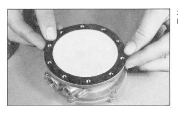
30. Place Gasket (15) in place and align with screw holes.
