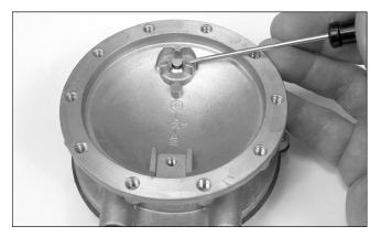
7. Gently lift up and remove the Valve Operating Pin (10).
