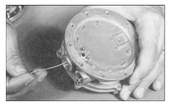
10. Insert paper-clip hook in center hole of Seal Retaining Washer (14) and remove.
