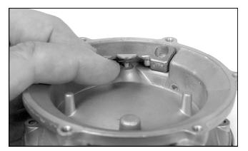
34. Lift Lever (6) to ensure it moves properly and verify that the Valve Pin (10) follows lever travel.
