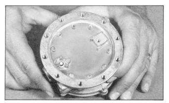
22. Pin (10) properly placed in valve jet.
